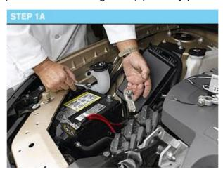
**STEP 1B:** Disconnect the red/positive (+) cable from the positive (+) battery post/bolt on the battery.
