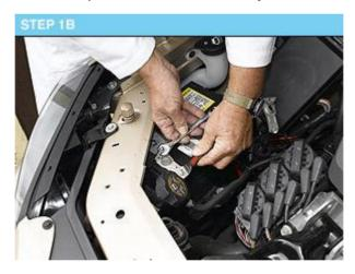
**STEP 2:** Connecting Battery Brain: With the Battery Brain in the "OFF" position, connect the positive (+) clamp to the positive (+) battery post.
