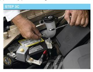
**TO COMPLETE INSTALLATION:** The manual reset control knob on the battery brain unit should be turned to one of the "ON" positions. Then press down on the manual reset control knob to establish contact.
