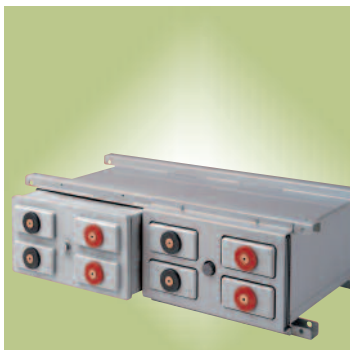
Absolyte GX – valve regulated lead-acid single cell batteries with a nominal capacity of 2000–6000 Ah at 25 °C. Maintenance-free (no topping-up).
